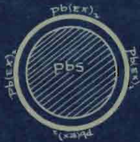
FIGURE 1Ba. LESS soluble xanthate film covers the easily soluble galena to make it float better.
